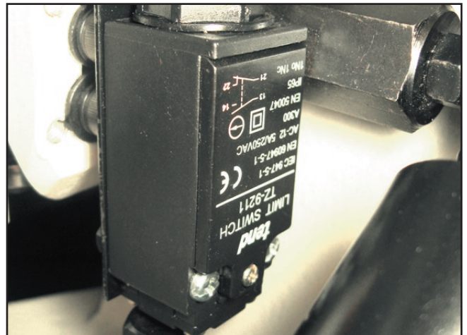
Figure 61. G0613 blade stop limit switch.
